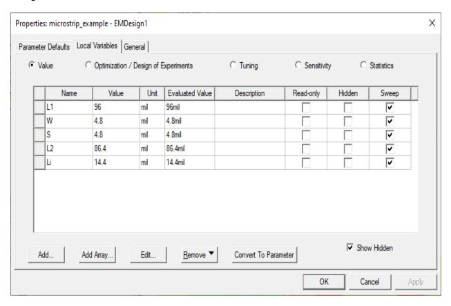
3. The **Local Variables** tab contains the variables that can be defined by the user, listed in the order in which they are defined. Enter a different number in the **Value** fields to alter the dimensions of the model, as chosen.
