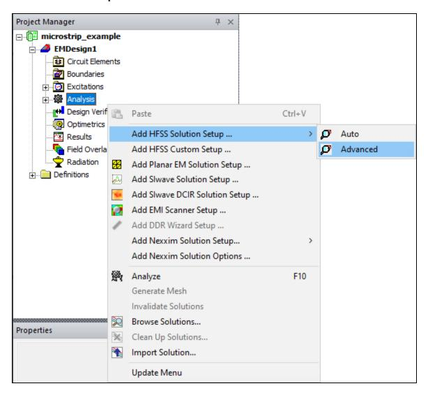
From HFSS 3D Layout, select Solution Setup > Add HFSS Solution Setup
