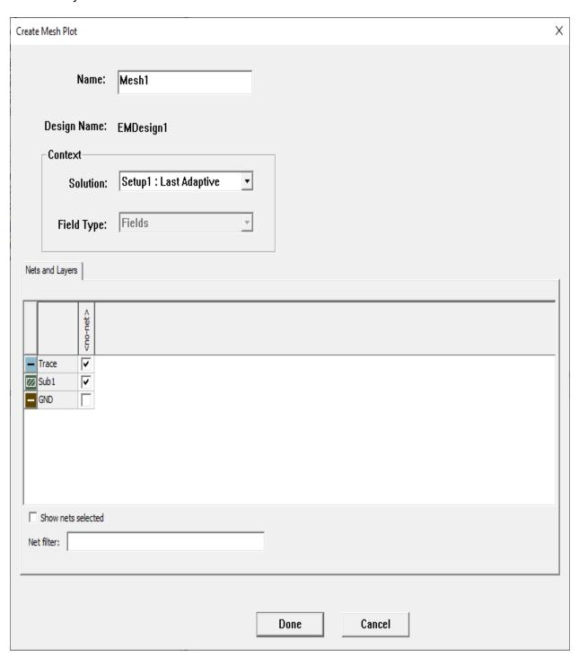
3. Click **Done** to close the **Create Mesh Plot** window and display the mesh for the **Setup1**: Last Adaptive solution in the Layout Editor.
