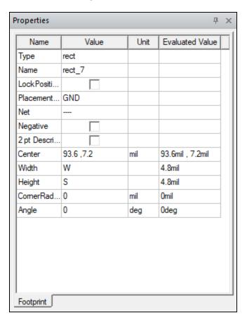
d. Enter **L1-W/2**, **W+S/2** in the **Center** field and press **Enter** or **Tab** to accept the coordinates.
