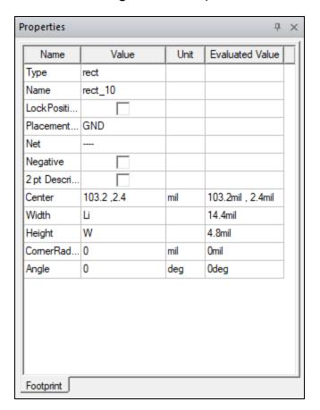
d. Enter **L1+Li/2**, **W/2** in the **Center** field and press **Enter** or **Tab** to accept the coordinates.
