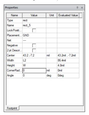
e. Enter **L2/2**, **-S-W/2** in the **Center** field and press **Enter** or **Tab** to accept the coordinates.
