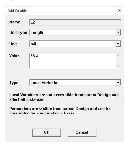
c. Select **mil** from the **Unit** drop-down menu and ensure **86.4** is entered in the **Value** field. Then click **OK** to close the **Add Variable** window.
