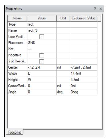
e. Enter -Li/2, W/2 in the Center field and press Enter or Tab to accept the coordinates.
