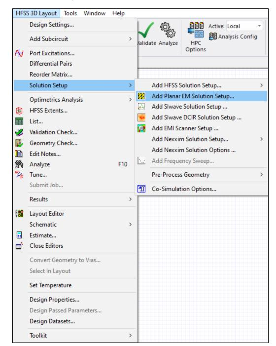
• From HFSS 3D Layout, select Solution Setup > Add Planar EM Solution Setup.
