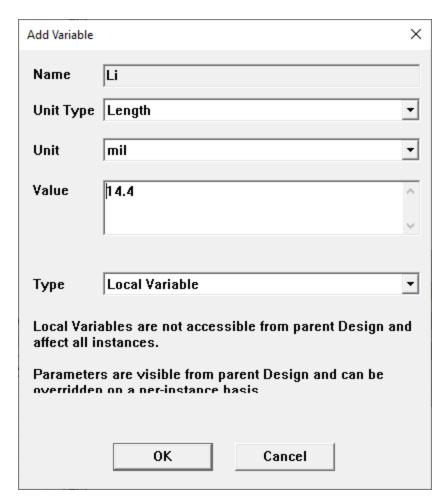
c. Select **mil** from the **Unit** drop-down menu and ensure **14.4** is entered in the **Value** field. Then click **OK** to close the **Add Variable** window.
