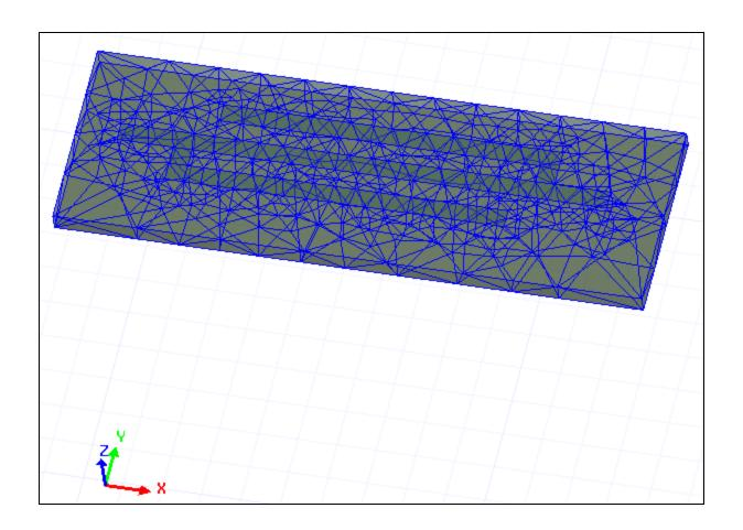
8. From the **Project Manager** window, right-click the mesh (e.g., **Mesh1**) and select **Plot Visibility** to remove the adjacent check mark and hide the mesh.
