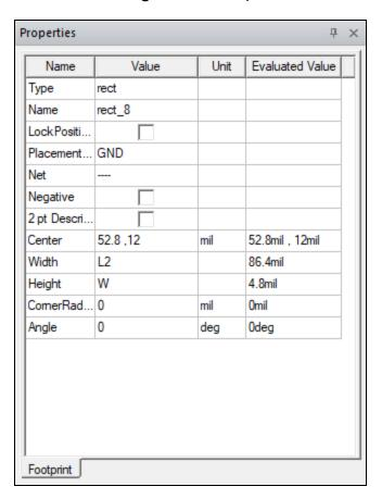
d. Enter **L1-L2/2**, **W+S+W/2** in the **Center** field and press **Enter** or **Tab** to accept the coordinates.
