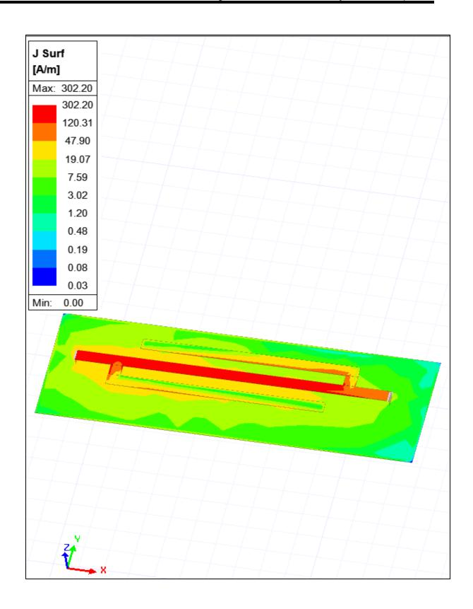
12. From the **Project Manager** window, expand **J Surf**. Then right-click **Mag\_SurfaceJ1** and select **Modify Plot** to open the **Modify Field Plot** window.
